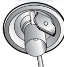
Inlet Valve with escutcheon being tightened into place with installation wrench
