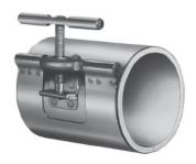
Quickon II Couplings for pnuematic or vacuum conveying systems can be installed or removed with the twist of the wrist. No tools or special skills needed. The positive-locking system turns easily to seal or to compensate for normal O.D. pipe or tubing tolerances.
