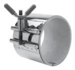
The Gripper Coupling was designed as a quick coupler for dry, bulk transport, tank tubing. This unique coupling just slides onto tubing or wraps around it and is tightented by hand in seconds but provides better support than rubber hose and band clamps.
