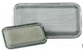
An aerator is a simple and efficient means of introducing low pressure air into any dry finely ground material. The air is equally distributed in controlled quantities to give the material an ability to flow by gravity from bins, hoppers or chutes. Aerators incorporate non-clogging diffusers, integral orifice and construction features which insure long, maintenance-free life.
