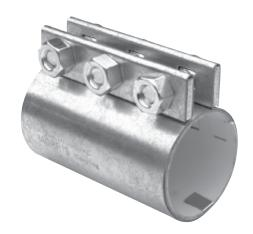
The Morris Compression tubing and pipe coupling is designed for permanent installation in the joining of either plain end, threaded, grooved or a combination of any of these joints. The band type construction holds the entire surface of the joint in uniform compression. Couplings are made of heavy-gauge zinc-plated steel. Prices of aluminum or stainless steel couplings quoted on request.
